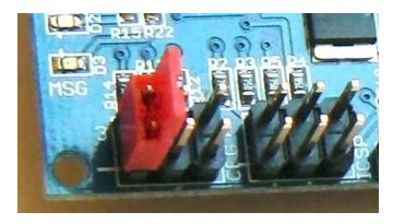
In Logic Level Commands mode, the pins CFG1 and CFG2 are trigger inputs. Pulling either pin low will activate the corresponding output switch (J1 and J2.) If activated by a short pulse, the output switches will stay active for one slide sensor cycle or about 819 milliseconds. If held low for a longer time, the switches will keep active until released and a sensor cycle completes or the timeout expires.
