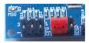
Note that this jumper is installed sideways, as opposed to the CFG jumpers which are installed vertically.
