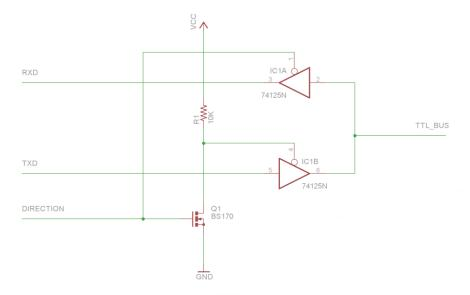
When transmitting data, set the direction control pin high, send the data as usual, wait for the last byte to be completely sent, and then set the direction pin low. The Dynamixel interface libraries that come with the OpenCM 9.04 board does this for you.
