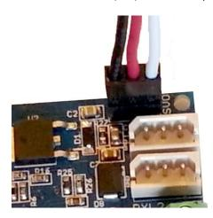
Similarly, when connecting the three-pin header to another board or controller, make sure to line up the black (ground) wire to ground (or negative.)
